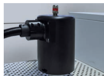
› Piezo Electric Injector
