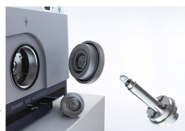
The exchange of the light source, if required, can be done in a few seconds. Also the desiccant cartridge, which keeps the inside low on humidity can be changed easily.
