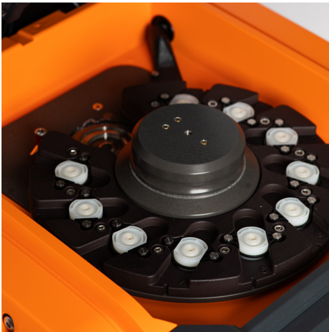
Figure 1. 10-position Autosampler Configuration 1
