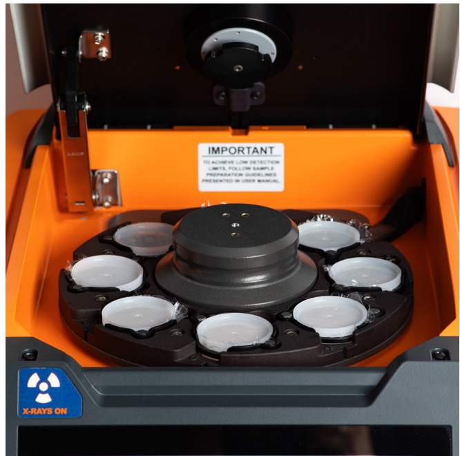
Figure 2. 8-position Autosampler Configuration
