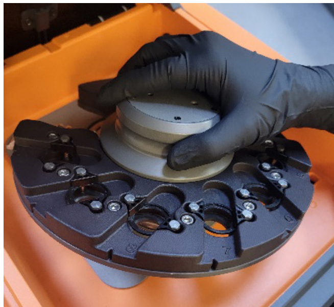
Figure 3. Autosampler Tray Removal
